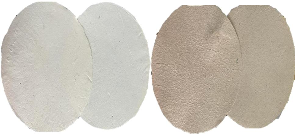
**Figure 10: Hand paper sheet from date palm residue before and after the bleaching process.**
