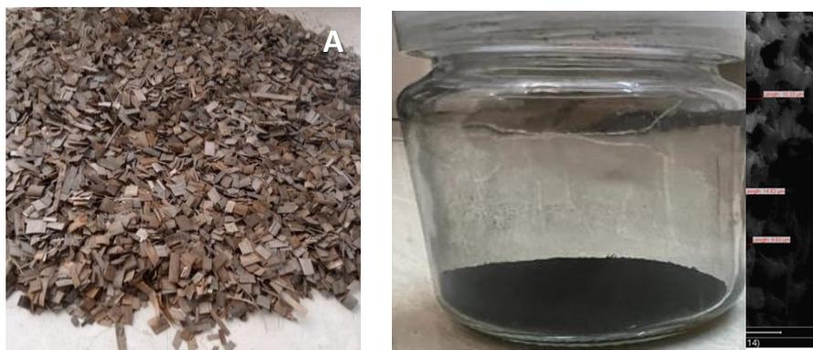
**Figure 4: Raw date palm leaves (A), activated carbon from date palm leaves (B), and SEM for prepared active carbon (C)**
